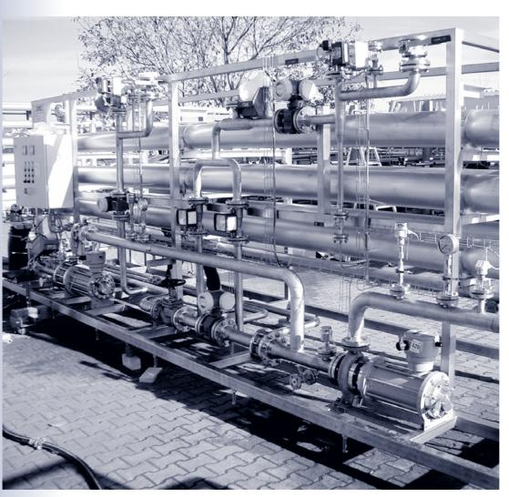
Together with the BFI Betriebsforschungsinstitut VDEh-Institut für Angewandte Forschung (Düsseldorf) and our customer ThyssenKrupp Nirosta (Dilenburg), OSMO Membrane Systems GmbH is developing a new environmentally friendly process for recovering valuable metal from stainless steel pickling using membrane electrolysis.
